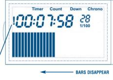
When the timer is in **COUNT UP** mode, the bars on the graphic display will fill in as time passes. When the timer is in **COUNT DOWN** mode, the bars will disappear as time passes.
